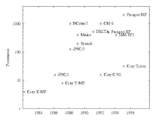
Number of processors in massively parallel computers (``o") and vector multiprocessors (``+"). In both cases, a steady increase in processor count is apparent. A similar trend is starting to occur in workstations, and personal computers can be expected to follow the same trend. *[source: Foster:3]*
