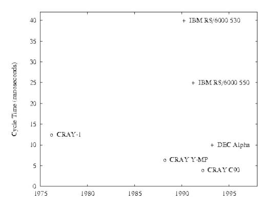
Trends in computer clock cycle times. Conventional vector supercomputer cycle times (denoted ``o") have decreased only by a factor of 3 in sixteen years, from the CRAY-1 (12.5 nanoseconds) to the C90 (4.0). RISC microprocessors (denoted ``+") are fast approaching the same performance. Both architectures appear to be approaching physical limits. *[source: Foster:3]*
