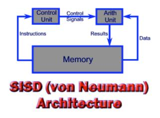
A central processing unit (CPU) executes a program that performs a sequence of read and write operations on an attached memory.
