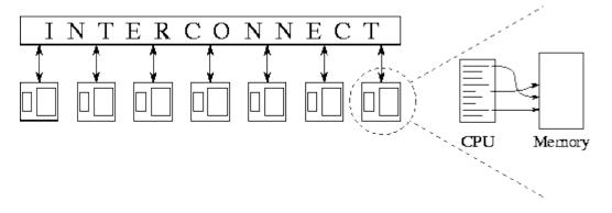
An idealized parallel computer model. Each node consists of a von Neumann machine: a CPU and memory. A node can communicate with other nodes by sending and receiving messages over an interconnection network. *[source: Foster:3]*
